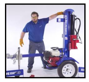
Use handle at top to lower the boom and secure the pin, see pictures below.
