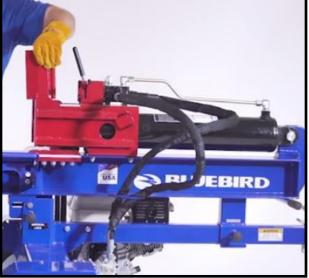
Insert splitting wedge and attach with bolt provided.
