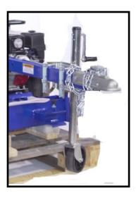
Rotate the jack to upright position and lower the wheel so the tongue will be level when installed.
