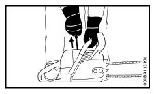
With the **first** recommended **method**, the chain saw is started on the ground. Make sure the chain brake is engaged (see "Chain Brake" chapter in your instruction manual) and place the chain saw on firm ground or other solid surface in an open area. Maintain good balance and secure footing.
