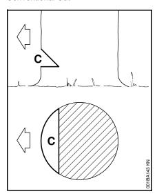
Felling notch (C) – determines the direction of the fall
