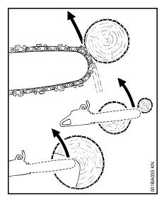
Kickback may occur, for example, when the saw chain near the upper quadrant of the bar nose contacts the wood or is
