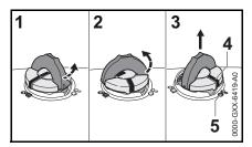
After allowing the chain saw to cool, remove the fuel filler cap slowly and carefully to allow any remaining pressure build-up in the tank to release:
