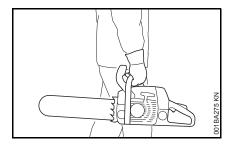
By hand: When transporting your chain saw by hand, the engine must be shut off and the chain saw must be in the proper position, i.e., grip the top handle and place the muffler away from the body; the chain guard (scabbard) should be over the saw chain and guide bar, which should point backwards, away from the direction in which you are walking.
