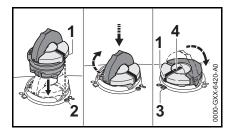
An improperly tightened fuel filler cap can loosen or come off and spill quantities of fuel. To reduce the risk of fuel spillage and fire from an improperly installed fuel cap, correctly position and tighten the cap in the fuel tank opening:
