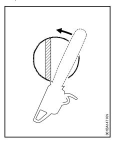
Engage the bumper spikes of the chain saw directly behind the location of the intended hinge and pivot the saw around this point only as far as the hinge. The bumper spike rolls against the trunk.
