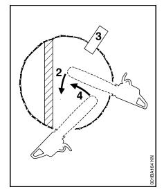
Avoid repositioning the saw more than necessary. When repositioning for the next cut, keep the guide bar fully engaged in the kerf to keep the felling cut straight. If the saw begins to pinch, insert a wedge to open the cut. On the last cut, do not cut the hinge.
