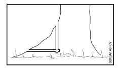
If the tree has large buttress roots, cut into the largest buttress vertically first (horizontally next) and remove the resulting piece.
