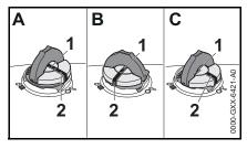
If the cap does not drop fully into the fuel tank opening when the positioning marks (1, 2) line up, or if it does not tighten properly when turned, the base of the cap may be prematurely rotated in relation to the top. Such misalignment can result from handling, cleaning or an improper attempt at tightening.
