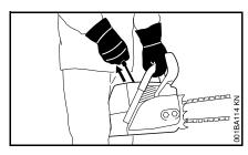
The **second** recommended **method** for starting your chain saw allows you to start the saw without placing it on the ground. Make sure the chain brake is engaged, grip the front handle of the chain saw firmly with your left hand. Keep your arm on the front handle in a locked (straight) position. Hold the rear
