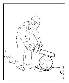
Bucking is cutting a log into sections.
