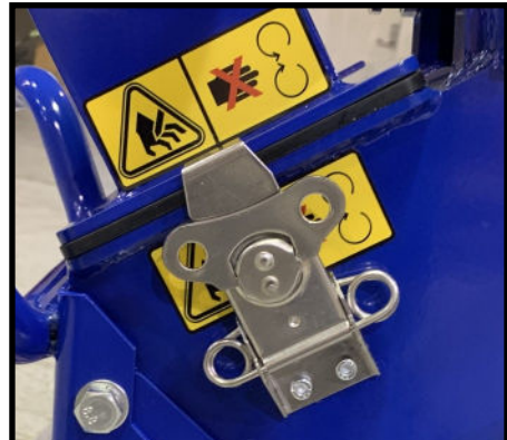
Latch both chutes by engaging in the chute, then turning the latch, then folding up the latch
