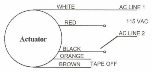
CONNECT THE WHITE & BLACK LEADS TO 115 VAC TO EXTEND. CONNECT THE WHITE & RED LEADS TO 115 VAC TO RETRACT. ORANGE & BROWN LEADS ARE NOT USED AND CAN BE TAPED OFF.
